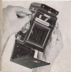
Inserting the empty take-up spool into the upper spool chamber
