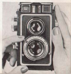
Tensioning the shutter for the self-timer (set the synchro-lever to "V")
