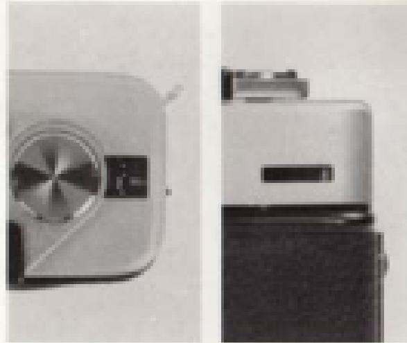
5. A large red dot should now appear opposite the red index in the frame counter window. Activate the film advance lever until it stops; then press the shutter release button. Repeat this lever actuation and shutter release until the number "1" appears opposite the counter index.
