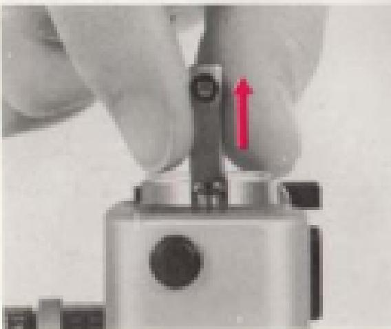
2. Place film cartridge into the film cartridge chamber. If film rewind key does not engage properly in end of cartridge, rotate film crank in either direction until it does so.
