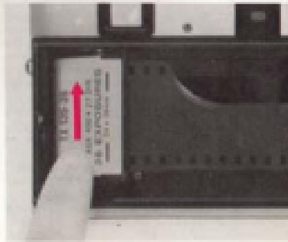
3. Insert leader of film about 3cm (1 1/2 in.) into one of the slots in the take-up spool. Be sure that a film perforation is engaged on a tooth of the slot.
