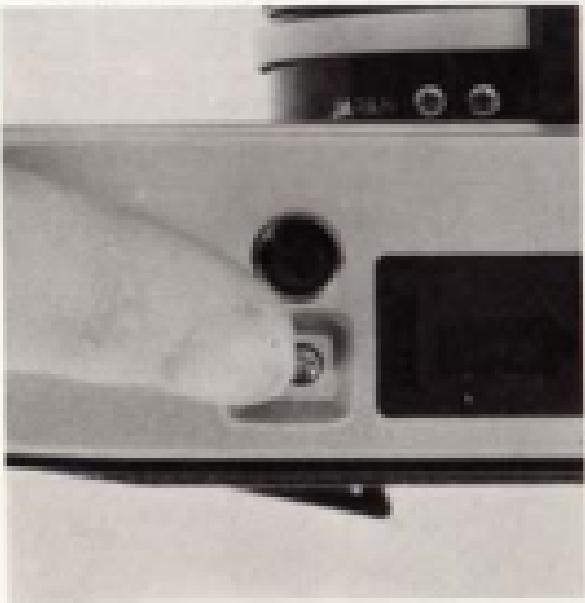
2. Lift the film rewind crank and turn it clockwise. This will rewind the film into the film cartridge. When all but the film leader is completely rewound and off the camera's spool, the red signal in the film load window will disappear. As you continue to turn the crank, you will feel a slight resistance. This means that the film leader is leaving the take-up spool. Continue winding a few more turns.
