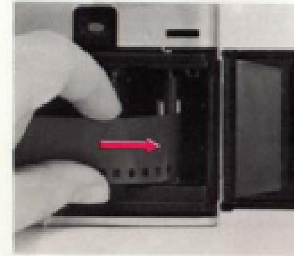
4. While pressing film gently against the sprockets, activate film advance lever slowly until the perforations on both edges of the film are engaged with sprocket teeth. Then close the back cover.
