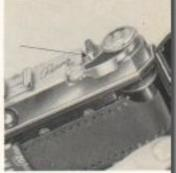
6. Press and release the film lever button (arrow in 5) and operate the film lever 3 times. Be sure to make a complete stroke with the lever; then let it fly back to its original position. This brings the first frame of film into place and cocks the shutter for the first exposure. It also brings the 36 or the 20 on the film counter into position.
