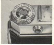
note: When the figure 1 in the film counter reaches the index, the film lever will lock; no more pictures can be made until the film is rewound into the magazine (see page 17) and the camera is reloaded. If the film lever locks at any time, do not force it but check the counter to see if it is set at 1. Move the counter off 1 to release the film winding mechanism.
