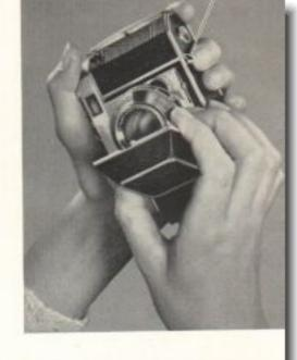
. . . this camera cannot be closed if it is focused for anything but infinity. Be sure the focusing knob is pushed clockwise, as you face the lens, as far as it will go; then squeeze the two CLOS-ING BUTTONS while
