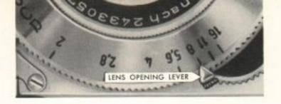
The opening is largest when the lever is set at 2 (f/2) and smallest when set at 16 (f/16). Each succeeding larger opening lets through twice the light of the one before; for example, f/8 lets through twice the light of f/11, and f/11 lets through twice the light of f/16.
