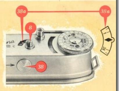
until the diamond-shaped mark • near Nr. 36 on the Film counter (38a) is opposite the notch in the upper edge of the film counter window. If you are using a 20-exposure cassette, set to the index mark • between No. 20 and 25. Now work the rapid-winding lever and press the film release button (8). Repeat this until the film counter indicates No. 36 or 20 respectively. At the same time the rewind knob (20) should rotate against its arrow if the film is advancing properly.
