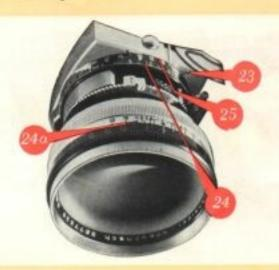
until the red dot is opposite the white dot on the bayonet ring. Before exposing with the telephoto lens measure the distance of the subject with the rangefinder and read off the distance. Transfer the measured value to the focusing scale for the telephoto lens (25). To do this turn the focusing knob until the appropriate distance on the telephoto scale is opposite T-index mark (23). Do not, however, use the black ring (25a) on the telephoto lens itself for setting the distances.
