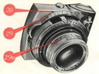
Set the distance in the same way as with the telephoto lens. Transfer the distance figure obtained with the rangefinder to the wide-angle distance scale (29) and read off from the mark (28). Always be sure to set the distance on the correct focusing scale when using the interchangeable lenses.
