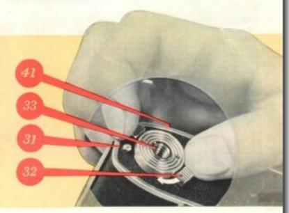
On the bottom of the camera you will find the tripod bush (33). This is surrounded by a double lever (32). If you push the milled end of the lever in the direction of the arrow, the opposite end uncovers a button (31). Depress this button, and the camera back (41) will spring open.
