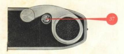
To rewind the exposed film depress the reversing button (37) in the base of the camera and half pull out the rewind knob (20) to get at it more easily. Then turn the rewind knob in the direction of the arrow until the reversing button ceases to rotate. This is easily observed by the small black dot near the rim of the button.
