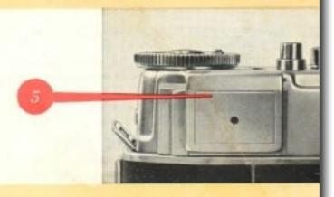
If the pointer of the exposure meter does not move appreciably with the cover closed, open the cover (5) by gently pressing on the ribbed upper edge. In this case read off the light value opposite the index mark (4a) for the open cover \*\*
