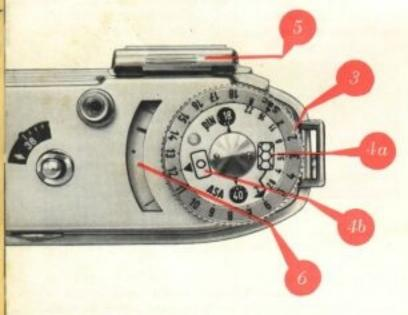
wards. A black pointer will move in the window (6). Turn the meter setting ring (3), thus moving a red pointer until the latter coincides with the black pointer of the exposure meter. If you have taken the reading with the cover (5) closed, read off the light value from the index mark (4b) \*\pi\$ on the setting ring (3)
